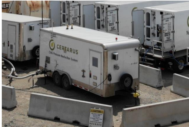
Portable CNG/RNG/Hydrogen Pressure Reduction Systems – Trailered pressure reduction systems for short and long-term deployment to customer delivery locations
