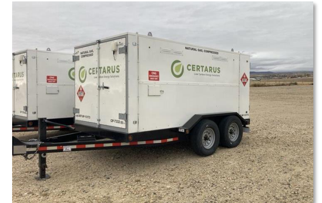
Small Volume CNG/RNG MSUs – Trailered mobile storage units with integrated pressure reduction systems for low-flow and backup gas supply applications
