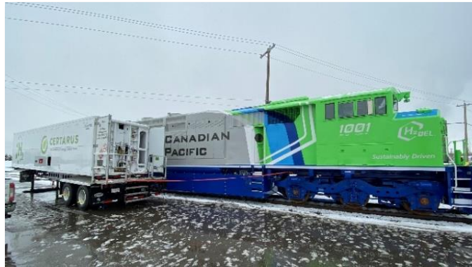
CP Rail: Supplied H2 for 3 Fuel Cell locomotives through commissioning and testing then for start up and commissioning of their electrolyzer facilities over 3 years
