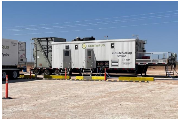
Portable CNG/RNG Compressors – Trailered gas engine-driven compressors capable of temporary assignment for filling MSUs for delivery
